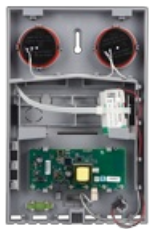
JA-163A-BASE-RB - bottom part with electronics
